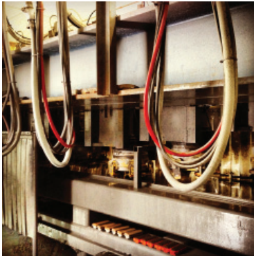
THE 8-HEAD GAUGER/ POLISHER USES DIAMOND BRICKS AND BRUSHES
