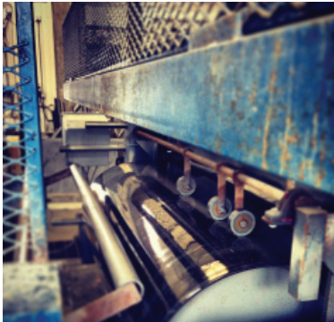
THE STRIP SAW RIPS SLABS TO WIDTH
