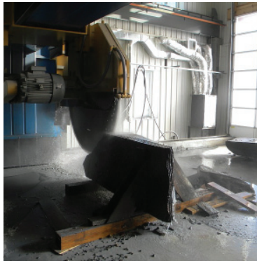
SLABS BEING CUT FROM BLOCK
