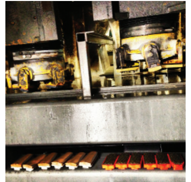
THE 8-HEAD GAUGER/ POLISHER USES DIAMOND BRICKS AND BRUSHES
