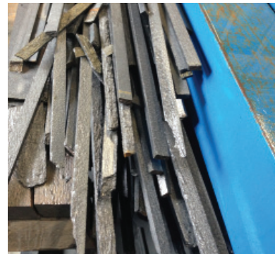
PLANKS AFTER SLABS ARE RUN THROUGH THE STRIP SAW AND RIPPED TO WIDTH
