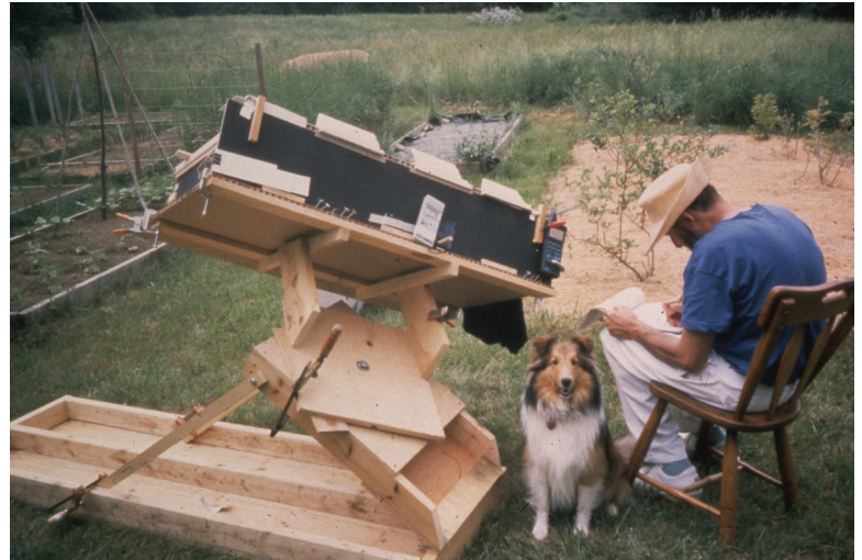
Daylight model testing of Stonyfield Farm office, Bruce Coldham & Skye Snuffles, 1995
