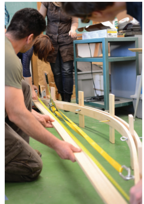
Proof testing: Bending capability of the laths
